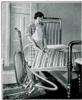
Fig. 4. — NETTOYAGE D'UN MATELAS A L'AIDE D'UN ASPIRATEUR A SAC MUNI D'UN RACCORD SOUPLE
