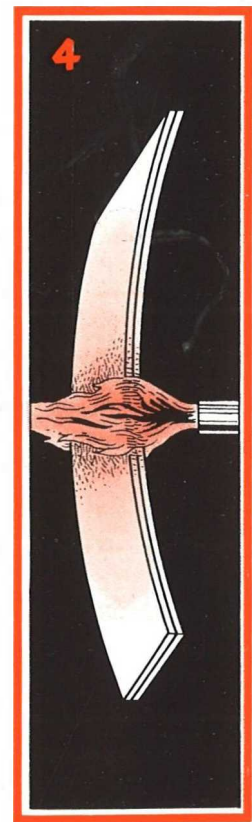
4 When heat is applied the Bimetal bends to a predetermined degree. When cooled it straightens!
