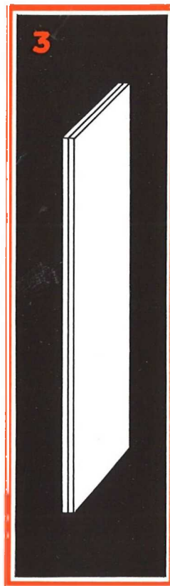
3 Both pieces of metal are joined together. The result is: BIMETAL .
