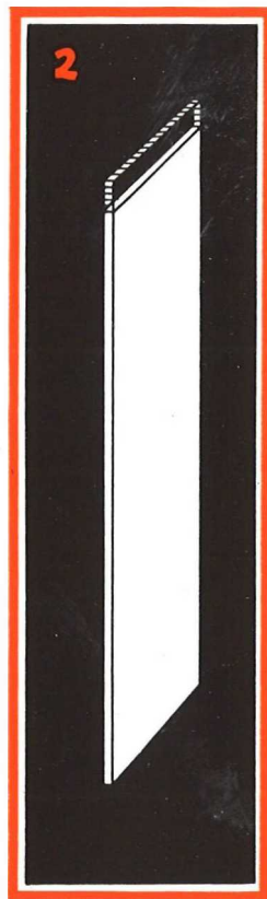
2 A piece of metal of LOW thermal expansion properties.
