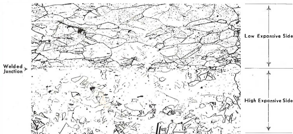
PHOTOMICROGRAPH OF CROSS SECTION OF CHACE THERMOSTATIC BIMETAL
