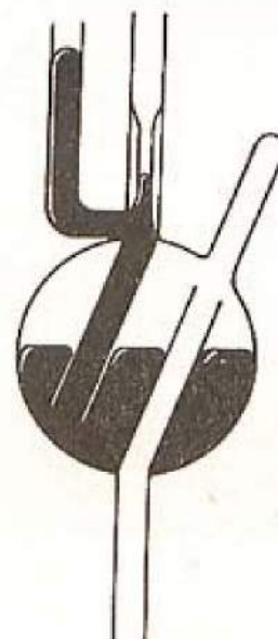
FIG. 8.—Arrangement to prevent creeping of toluene to mercury contact-surface.
