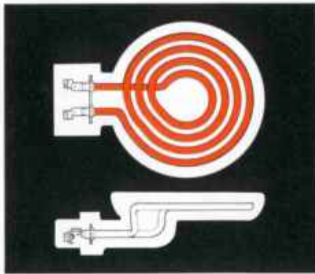
6D1/245/4 (registered design applied for) 1500W. 6" diameter – 4 turn – single circuit. With twin tab and screw terminals. Use – replacement for 6D1/2, 6D1/4, 1500W and 6D1/5 1000W.
