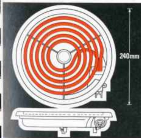
SS220D 2200W. 220mm (9" nominal) diameter – 5 turn – single circuit lift-clear swivel element. With tab terminals and deep reflector.
