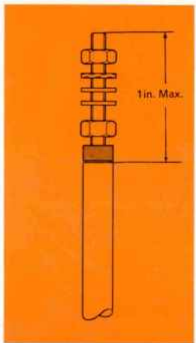
Code 1727 Title 4BA Screwed Terminal Max. Temp. Mild Steel Plated 325°C Stainless Steel 500°C
