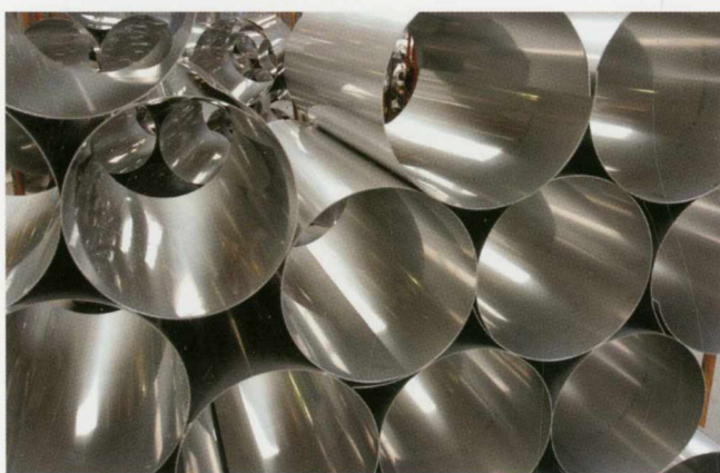
Rolled sheets of stainless steel await welding in ACV's Belgian factory
