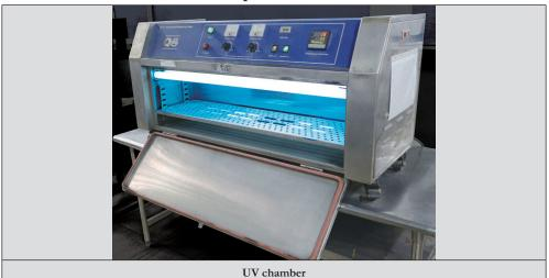
1000 hours UV resistance testing, made in our laboratory, on plastic specimens
