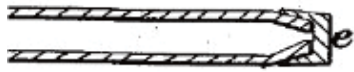
1847 Fusible plugs on boilers of steam locomotives. Cap "e" melts and releases steam (US patent # N°5022, Alfred Stillman)
