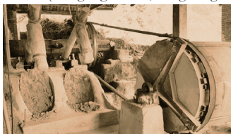
Traditional production machines ((水碓 shui duì) for production of powders used to make electric porcelain (private collection)
