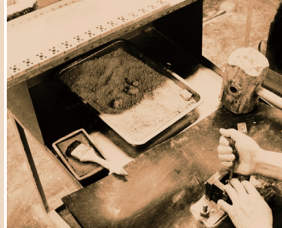
Porcelain Terminal Blocks Hand Made by Hammer Pressing: Manual Filling of Wet Granulate (Private Collection) Drying of Electric Porcelain After Pressing (Private Collection)
