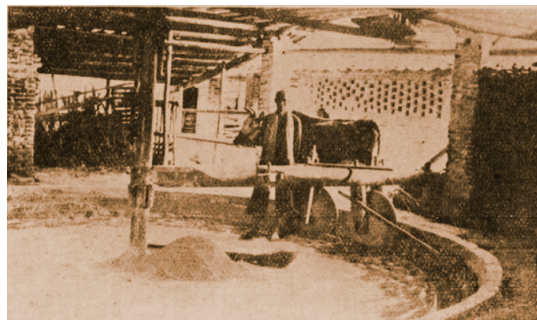
Grinding of kaolin by grinders powered by an ox (1939, Vietnam, Economic Bulletin of Indo-China)
