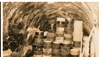
Traditional Chinese Dragon oven (龙窑 Long Yao), feeding mouth and filling method with electric porcelains (private collection)
