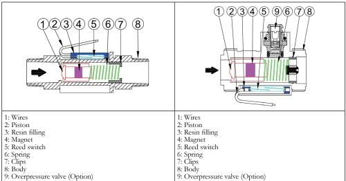
**Piston and reed switch types** Piston type flow switches place a piston directly <u>in 100% of the flow path</u>.
