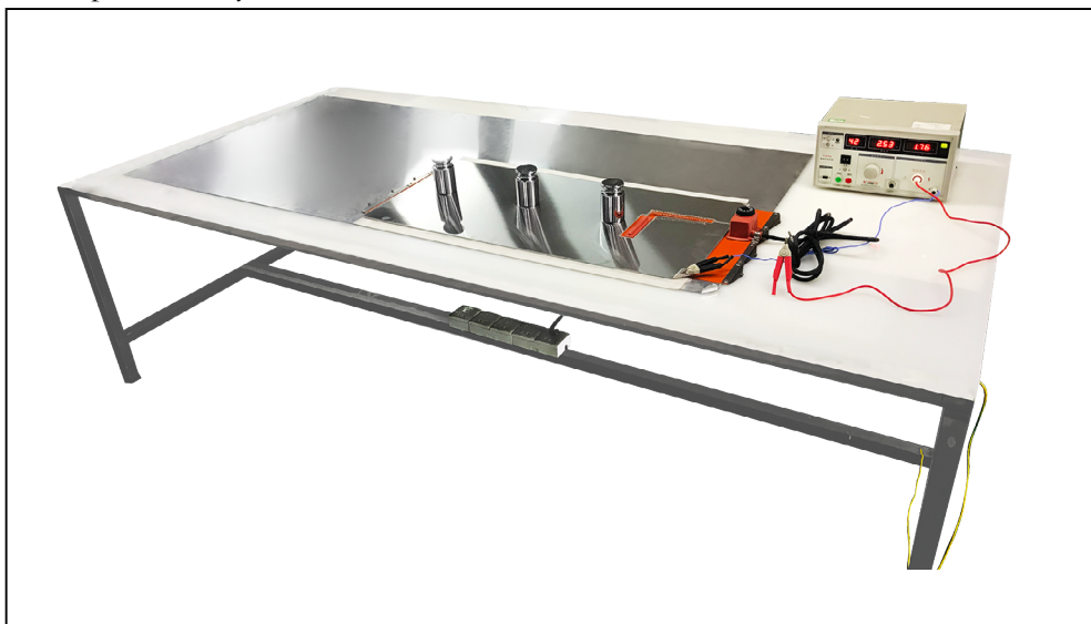
Measuring equipment for total current leakage at cold condition
