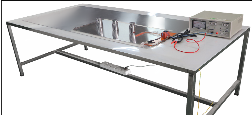
Device for measuring the insulation resistance. The measured values are always greater than 0.1Gohm
