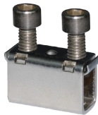
Stamped terminal with clamping screw and pressure plate (Used on ceramic terminal blocks with large sections or to withstand very high temperatures)
