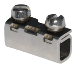
Stamped terminal with direct clamping screw (Used on ceramic terminal blocks with large sections or to withstand very high temperatures)
