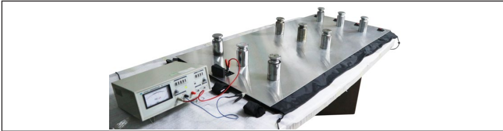
Device for measuring the insulation resistance. The measured values are always greater than 0.1Gohm
